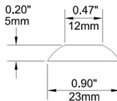
Figure 1. Dome Section
