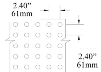
Figure 2. Dome Spacing
