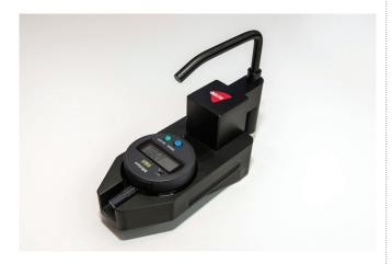
DELTA's Marking Thickness Gauge is a digital devise for measuring the thickness of pavement markings dry, after application. The Marking Thickness Gauge is very easy to operate and comes in a sturdy construction and ergonomic design. The Marking Thickness Gauge can measure markings within the measurement range of -12.7 mm to +12.7 mm / -0.5 inch to +0.5 inch. The digital display provides reliable measurement results in seconds.
