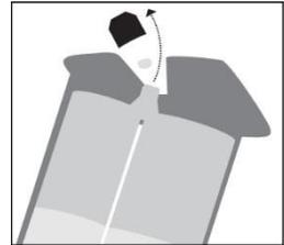
Figure 5: Remove nose plug with gun upright
