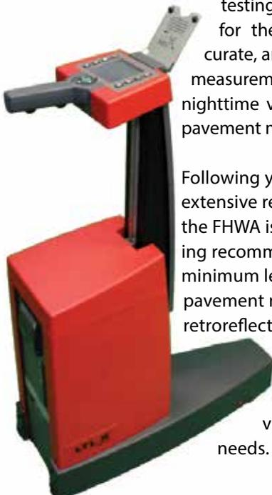
The LTL-X Mark II is an important component to properly measure and verify data when implementing any of the proposed maintenance methods. DELTA instruments are repeatable, reproducible and traceable to a NIST national standard through an ISO 17025-certified testing and calibration laboratory.
